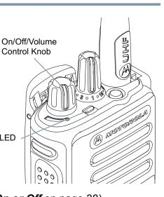
If your radio does not power up, check your battery. Make sure that it is charged and properly attached. If your radio still does not power up, contact your dealer.
