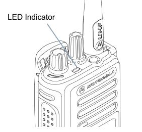
**Blinking red** – Radio is transmitting at low battery condition, receiving an emergency transmission, has failed the self-test upon powering up, or has moved out of range if radio is configured with Auto-Range Transponder System.
