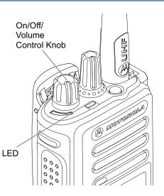
NOTE: The Home screen does not light up during a power up if the LED indicator is disabled (see *Turning the LED Indicator On or Off* on page 101).
