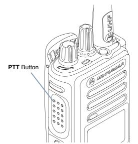
• While a call is in progress, the **PTT** button allows the radio to transmit to other radios in the call.
